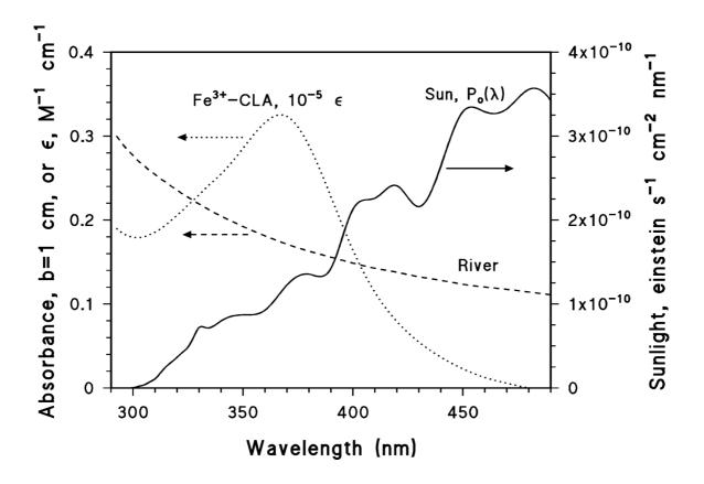
Fig. 7: Molar absorption coefficient of  $\text{Fe}^{3+}$ -CLA, absorption spectrum of river water for an optical path length b = 1 cm, and emission spectrum  $P_o(\lambda)$  of sunlight under summertime irradiation conditions (clear sky, noon, mid-latitude; Frank and Klöpffer, 1988).
