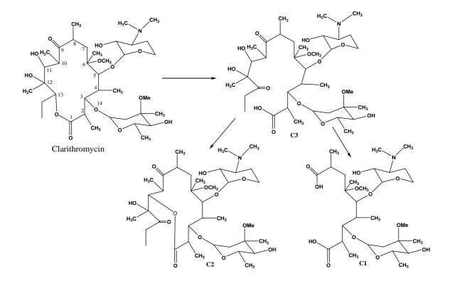
**Fig. 5:** Possible phototransformation pathways of clarithromycin in water in the presence of Fe(III), under UV-Vis lamp irradiation.
