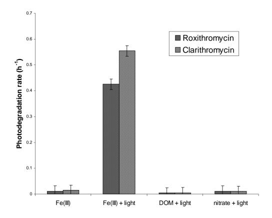
**Fig. 3:** Photodegradation rate constant (h<sup>-1</sup>) of human-used macrolides under UV-Vis lamp irradiation and different experimental conditions.  $[ML]_0 = 1.34 \ \mu\text{M}$ ;  $[Fe^{3+}] = 37.7 \ \mu\text{M}$ ;  $[NO_3^{-1}] = 0.8 \ 10^{-3} \ \text{M}$ ;  $[DOM] = 10 \ \text{mg/L}$  (humic acids).
