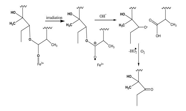
**Fig. 6:** Mechanism of cleavage of the lactone ring in the presence of Fe(III) and under UV-Vis lamp irradiation.
