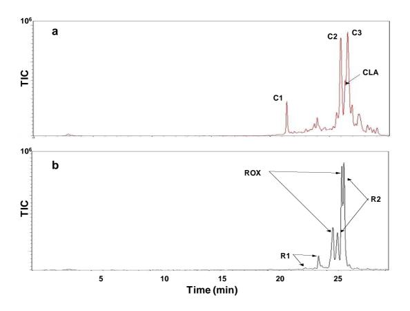
**Fig. 4:** Typical total ion chromatograms (TIC) showing the separation a) of three photoproducts of clarithromycin, C1, C2 and C3 and b) of two photoproducts of roxithromycin, R1 and R2.
