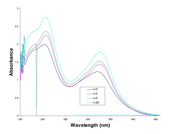
**Fig. 2:** Overlaid UV spectra of FeCl<sub>3</sub> titrated with Clarithromycin.  $[Fe^{3+}] = 4.46 \ 10^{-5}$  M; r is the mole ratio of ML to metal; solvent methanol:water (50:50, v/v); pH 7. Plots of the data in the form of the Scott equation in insert.
