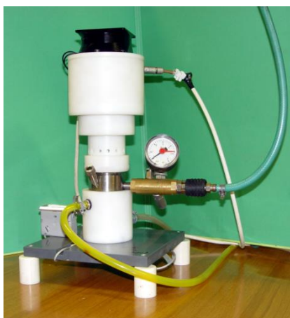
Figure 2a. A water cooled horn-type US-reactor to work under pressure (up to 7 bar).
