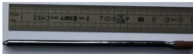
Fig. 1. As grown CaFeO 2.5 single crystal obtained by the floating zone method
