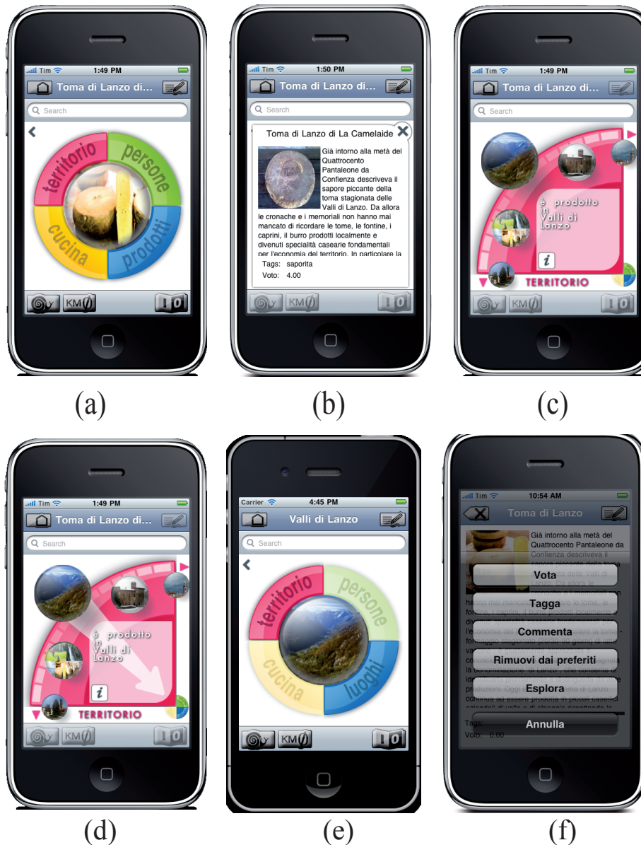
Fig. 2. Example of the wheel on the iPhone. (a) The wheel with the thing in focus in the center and the four sectors (“Persons”, “Products”, “Cuisine”, “Region”). (b) Getting details about the thing in focus. (c) Exploring one of the sectors of the wheel; the friends of the thing in focus are shown displayed as small circles in a ring. (d) Selecting one item from the sector and dragging and dropping it to the center of the wheel (shown as an icon in the bottom right corner). This leads to a new wheel (e) with the selected item in the center. (f) User’s possible actions on the things in focus (“Vote”, “Tag”, “Comment”, “(Add To/Remove From) favorites”, “Explore”).
