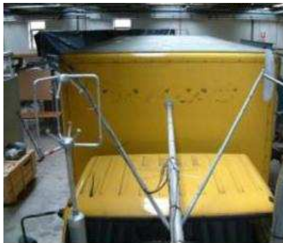
Figure 6: Front view. Front tapping points, anemometer
