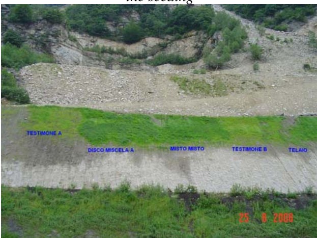
Figura 3.a: “Cava del Tiglio” Loc. Pra del Torno, in Rorà Village (TO), in this area it was used a “artificial loam” (mix A, C and D) compared to natural soil. The rehabilitation at the bottom is realized using only compost from ACEA (June 2008)
