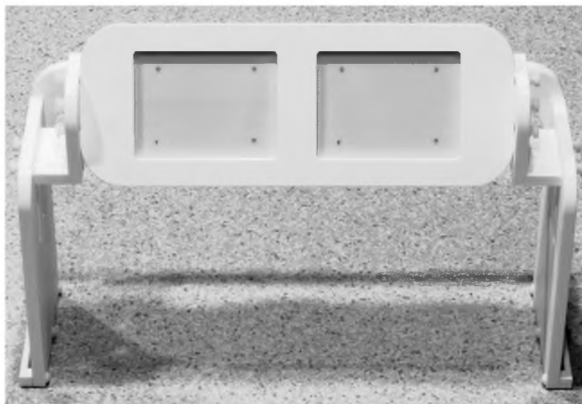
Fig. 2. Dual panel fMRI-compatible tablet.
