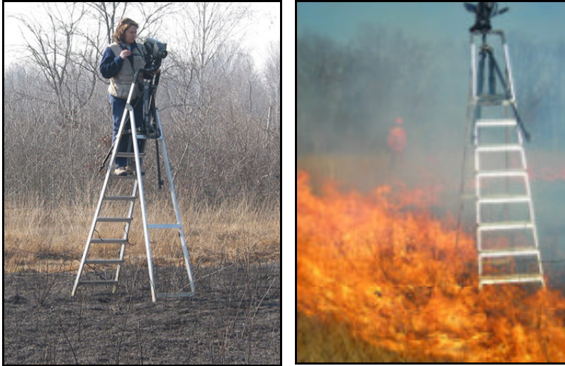
Figure 4-16 Infra Red Camera filming a head fire temperature residence profile.
