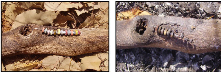
Figure 5-13 Sets of thermo sensitive crayons placed on a log
