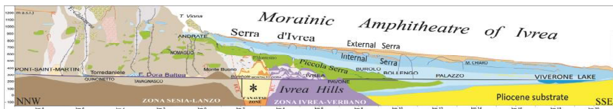
Fig. 5 - Longitudinal profile of the Ivrea Amphitheatre with the Serra of Ivrea morainic group. The Serra d'Ivrea is morphologically divided into External Serra (brown) and Internal Serra (blue). A deep glacial excavation hollow in correspondence of the Canavese Zone bedrock (black asterisk), whose bottom is below sea level, was discovered by means of a 270 m deep coring at Montalto Dora. The Ivrea Hills represent the threshold by which the Aosta Valley is perched above the Po Valley.
