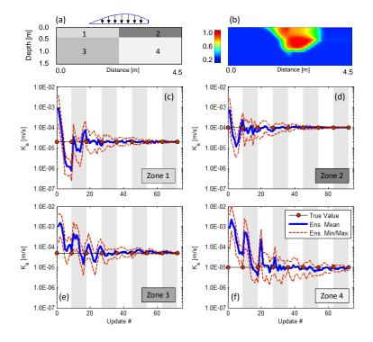
Figure 6: Heterogeneous test case results: (a) conceptual model of the model domain (divided into 4 zones with different soil properties) and (b) the simulated soil saturation at t = 5.5h. Convergence of the hydraulic conductivities of the four zones is shown in panels c-f. The results are relative to  $\sigma_{\Phi} = 5\%$  with randomly perturbed measurements.
