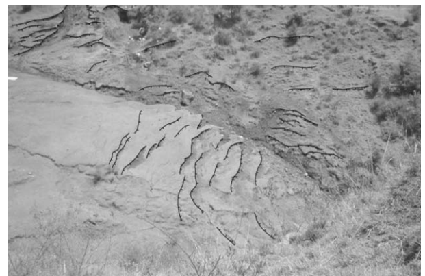
Fig. 5. Rotational slides in lacustrine sediments with crescent shaped fractures.
