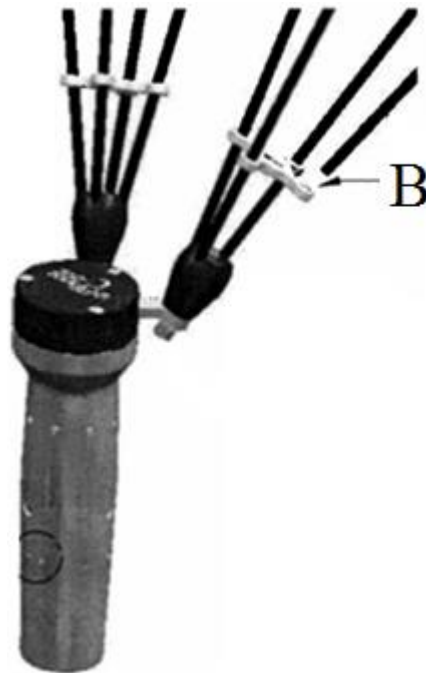
Figure 8 – Graphical instructions for the mounting of the anti-breaking devices (extracted from the beater user manual)
