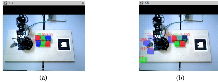
Fig. 5. Scenarios with different similarity thresholds for the object recognition algorithm. Thresholds are set to 90% in (a) and 85% in (b). Comparing with Figure 1, in (a) objects are recognized and added to the KB. For the case of (b) false positives are introduced by decreasing the threshold.
