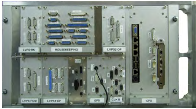
Fig. 4 The Data Processor (DP) collects and processes the data from the PDM. It handles their on-board storage, and sends a subset to the telemetry system. The DP also includes the housekeeping system. The various sub-assemblies are contained in an aluminum crate to assure thermal contact with the radiator.
