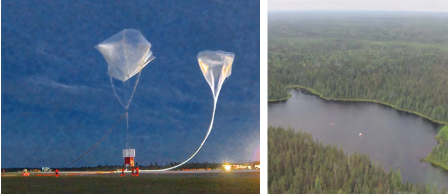
Fig. 9 left: Timmins (Ontario, Canada) Stratospheric Balloon Base, August 25, 2014, 0:53 UT : the perfect launch of EUSO-Balloon by the balloon division of the French Space Agency CNES, the auxiliary balloons (above the payload in the picture) warrant a smooth launch even in case of moderate surface winds. right: the instrument floating in the middle of “Lake Euso” after splashing down at 8:59 UT. All systems survived the impact and more than eight hours in the water thanks to a dedicated “water-landing” design.
