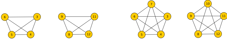
Figure 2: Illustrative example for the CNP3 b (with N = 2 ) where using GR2( S, 3, b ) in the graph in Fig. 1 deletes unnecessary nodes, namely nodes 7 and 10 (on the left). The sequential use of GR1( S, 3, b ) right after reintroduces nodes 7 and 10 in the graph thus yielding an optimal solution (on the right).
