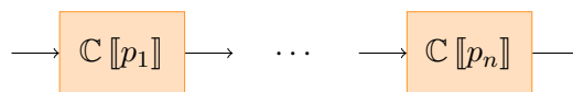
(B) \mathbb{C} [p_1 \mid \dots \mid p_n] = \mathbb{C} [p_1] \circ \dots \circ \mathbb{C} [p_n]
