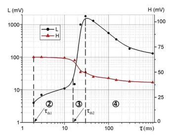
Fig. 3. Photomultiplier output, L, and hydrophone output, H, versus ultrasound pulse duration,  $\tau$ , at ultrasound pulse period T = 100 ms: Up-p = 150 V,  $\theta$  = 23  $\pm$  1 °C.
