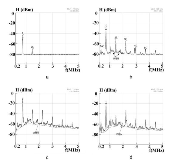
**Fig. 6.** Cavitation noise spectra at different stages of cavitation zone development in the focused ultrasound field: (a) stage one, below SL threshold; (b) stage 2, from SL threshold to a sharp increase in SL intensity; (c) stage 3; (d) stage 4. Pulse period T = 30 ms, pulse duration  $\tau$  = 3 ms,  $\theta$  = 23 ± 21 °C.
