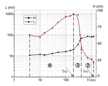
**Fig. 4.** Photomultiplier output, L, and hydrophone output, H, versus ultrasound pulse period T at a pulse duration of  $\tau$  = 5 ms: Up-p = 150 V,  $\theta$  = 23 ± 1 °C.
