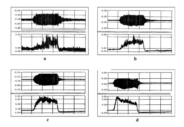
**Fig. 5.** Hydrophone output H (upper diagram in every pair) and photomultiplier output L (lower diagram in every pair) at the different stages of cavitation zone development: (a) the end of stage 1; (b) stage 2; (c) stage 3; (d) stage 4. T = 30 ms,  $\tau$  = 3 ms, Up-p, V = 105 (a), 175 (b), 210 (c) and 255 (d),  $\theta$  = 23 ± 1 °C.
