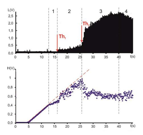
**Fig. 2.** Simultaneous recording of SL intensity L (upper panel), and hydrophone output H (lower panel), T = 30 ms,  $\tau$  = 3 ms,  $\theta$  = 23 ± 2 °C. The oscilloscope was operated in peak mode. Cavitation zone stages are separated by dashed vertical lines.
