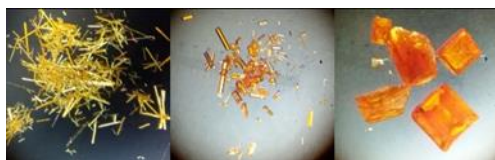
Figure 5. Single crystals of compounds 12·I2F4 (left), 22·I2F4 (middle) and 32·I2F4 (right), obtained by recrystallization from solution of the mechanosynthesis products (see Experimental).
