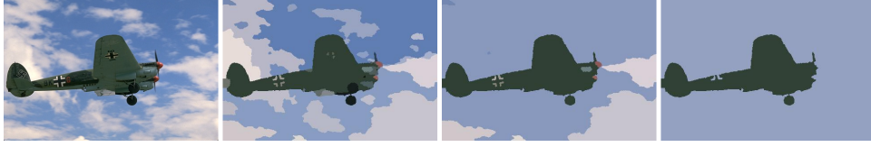
FIGURE 6.2: A sample image and hierarchy of 3 segmentations obtained with k = 50, 15, 2 and \delta_C metric.
