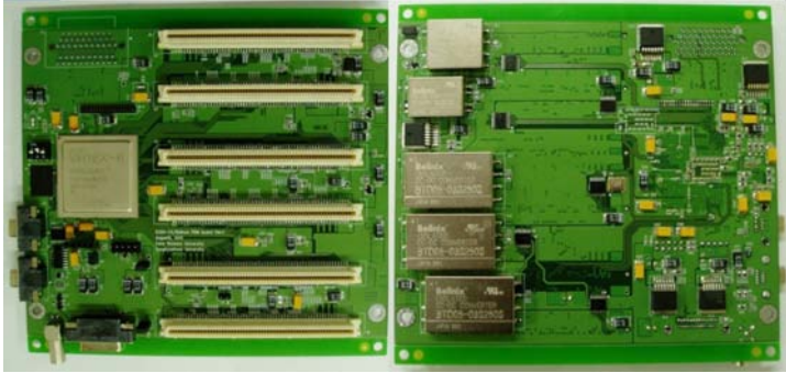
Fig. 15 PDM board, responsible for reading 36 MAPMTs through 6 EC-ASIC boards (white slots visible on the picture on the left) and performing real-time trigger.
