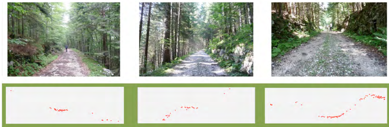
Figure 44: Example of the density and the distribution of the ground points used to extract the forest cross-sections below forest canopy
