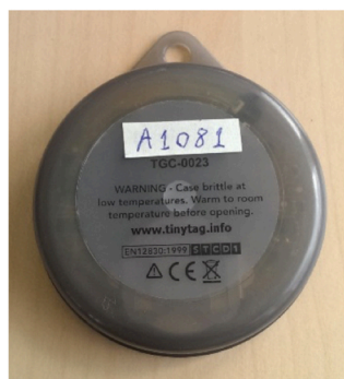
Fig. 2. TinyTag Transit 2 temperature data logger (a) and Watts Up PRO electricity consumption meter (b).
