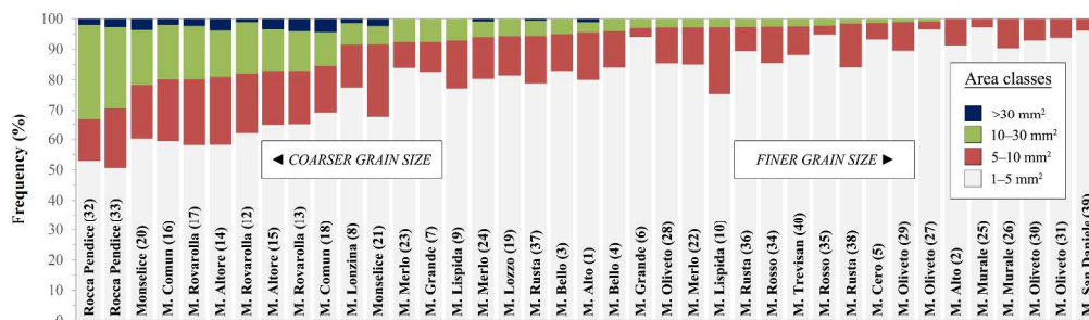
Frequency histogram of size classes of feldspars expressed as area, determined by DIA of \mu -XRF maps for each trachyte quarry. Quarries are indicated with locality name and ID number in parentheses.
