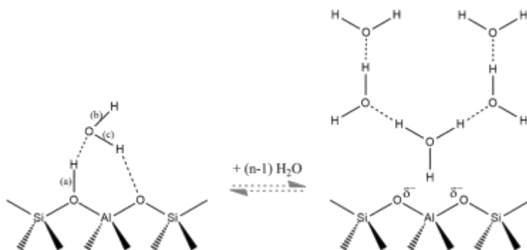
Scheme 3 Evolution of hydrogen bonded 1:1 \text{H}_2\text{O}/\text{H}^+ adducts into n\text{H}_2\text{O}/\text{H}^+ with n > 1 , implying deprotonation and presence of \text{H}_2\text{O} clusters
