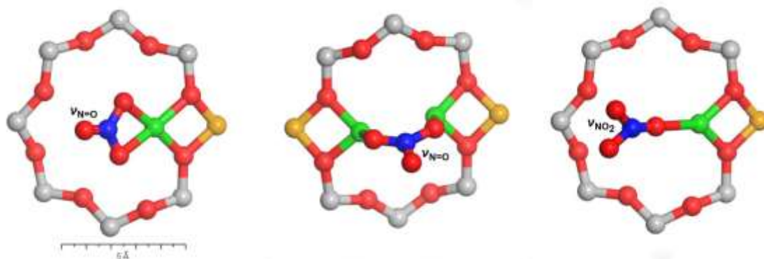
Scheme 2. Pictorial representation of the structure of different \text{Cu}^{\text{II}}\text{NO}_3^- complexes involving \text{Cu}^{\text{II}} ions in the chabazite 8-member ring: chelating bidentate (left), bridging bidentate (middle) and monodentate (right). Cu: green, Si: white, Al: yellow, O: red and N: blue. The labels \nu_{\text{NO}_2} and \nu_{\text{N}=\text{O}} indicate the corresponding vibrational modes observed and discussed in this work.
