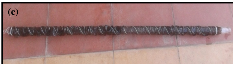
Fig. 1 – (a and b) Compound Parabolic Collector reactor (c) Inner tube coated with the CHIT- CNP composite film
