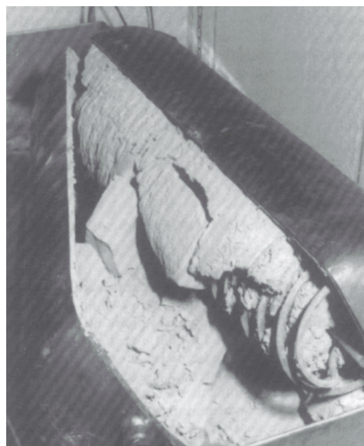
Figure 36. Left: layout of \text{MgH}_2 tank for a process steam generator. Right: The tank opened after 1.5 years of operation [345].
