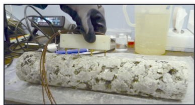
(a) Electrical resistivity measure on a macrocrystalline gypsum sample
