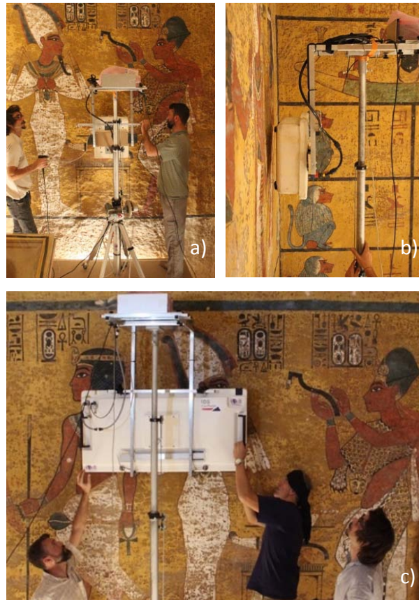
Figure 3: Pictures taken during LF and IF radar scans showing: a) and b) the IDS TR200 shielded antenna and c) the multi-channel IDS Stream-C system deployed by the lifter.
