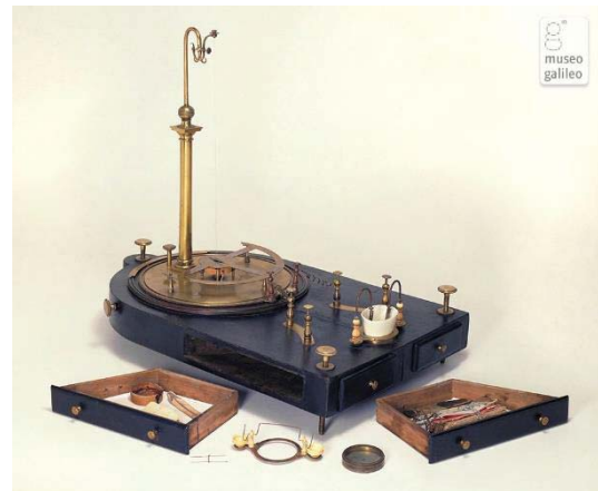
Fig. 1. Nobili's astatic galvanometer (Institute and Museum of the History of Science, Florence)
