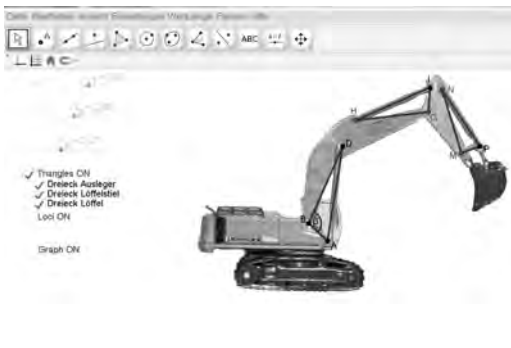
Fig. 5 - A digital simulation of the excavator
