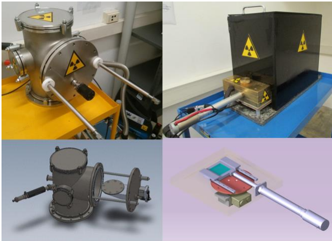
Figure 1. On the left: \alpha -irradiation system with a view of the inner sample-holder wheel. On the right: \beta -irradiation system and a scheme of its internal structure.
