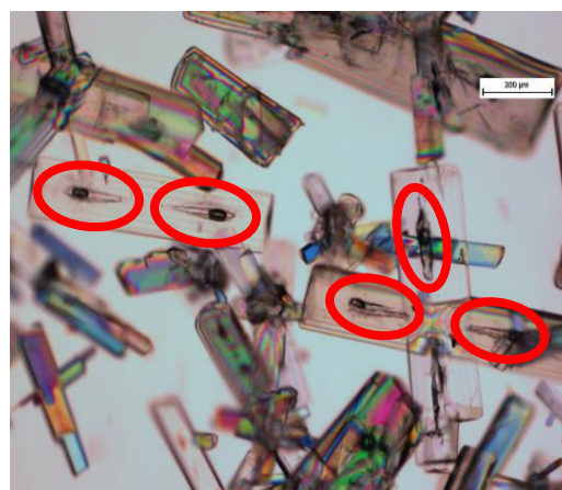
Figure 1: Encircled in red the symmetrical fluid inclusions obtained in a mixture: ethanol–Water (80-20%) and a supersaturation: \beta = 1.8 at 20°C; seeding at 40°C.
