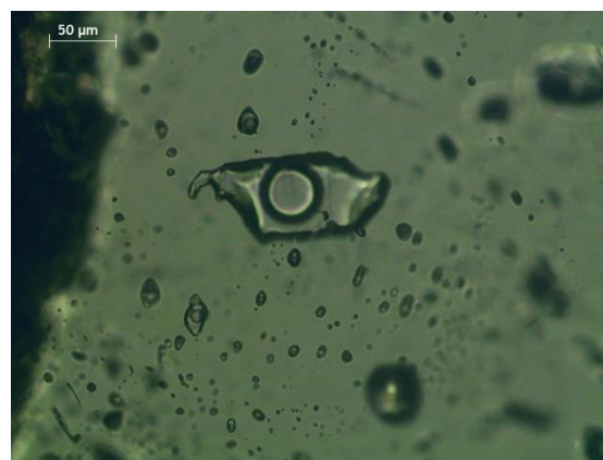
Fig. 1: Isolated primary fluid inclusion in scheelite. Objective 5x. In the back, other primary isolated FI and intra-granular trails of pseudo-secondary FI.
