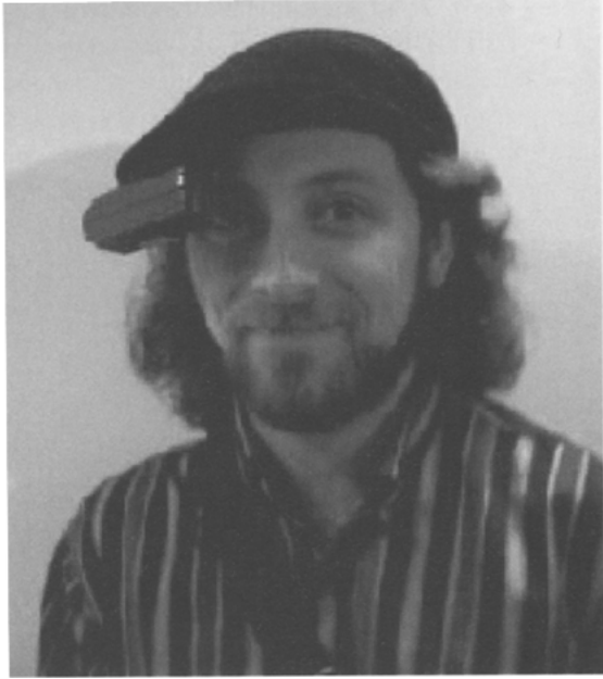
Figure 4. The heads-up display for the wearable platform. Reprinted by permission from Springer Nature: Springer Nature, Personal Technologies , The wearable remembrance agent: A system for augmented memory, Rhodes, B. J., Copyright (1997) by the publisher.
