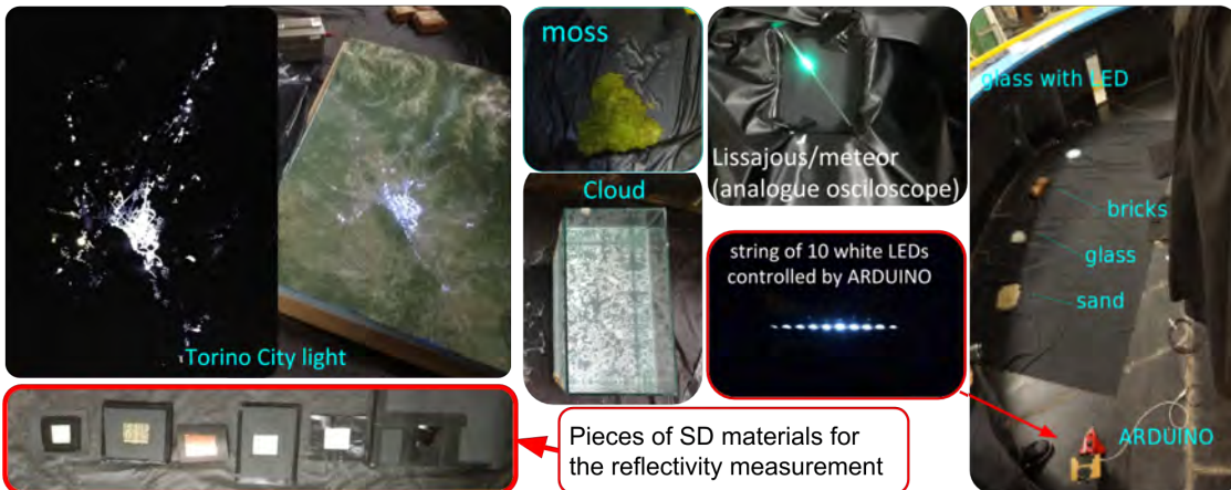
Figure 4: Light sources and materials to reproduce phenomena that Mini-EUSO can observe are visible. Reflections of materials that are often present in space debris (SD) have also been tested.
