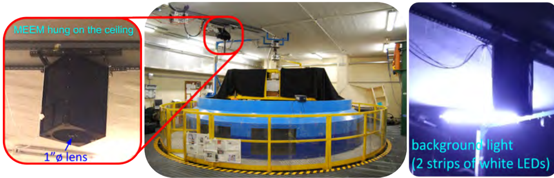
Figure 3: The TurLab tank setup with the Mini-EUSO EM installed on the ceiling and enlarged inside the red frame (left). The diffused airglow in the atmosphere was represented with two strips of cold-white LEDs reflected by the ceiling above the tank (right).
