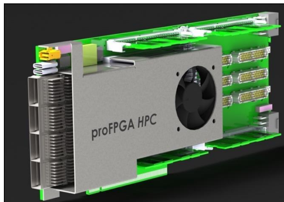
Figure 12. The new DeepHealth FPGA board optimized for inference operations.
