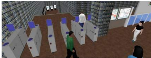
Fig. 1. The microsimulation model (faregates detail).
