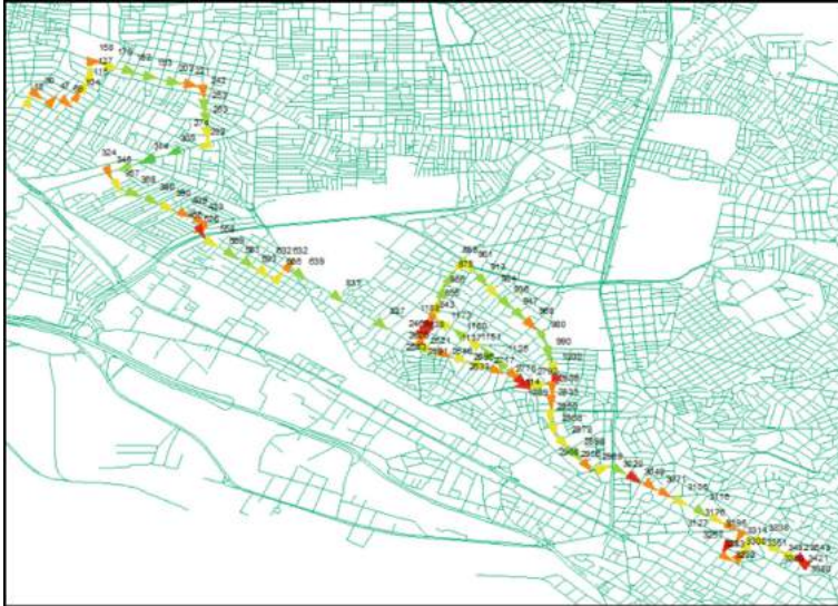
Fig. 2. Sample of floating car data in the city of Thessaloniki (one vehicle, one hour).
