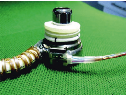
■ Fig. 31.6 Reduction of the effective length of the inflow cannula with two Dacron velour-covered 5 mm silicon suture rings
