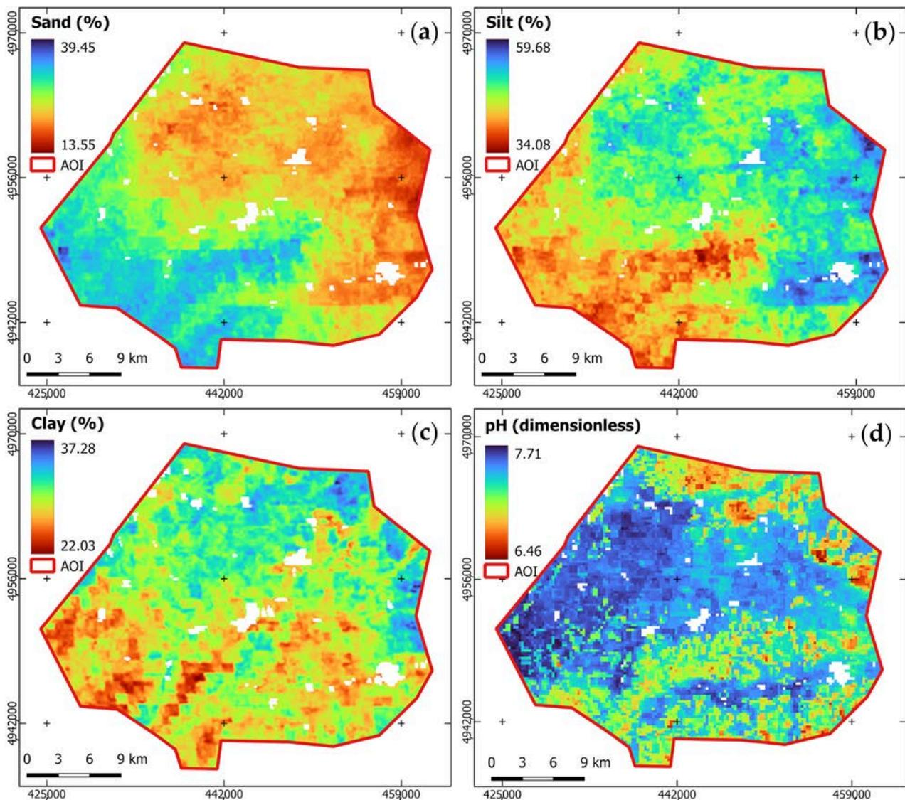
**Figure 5.** Raster layers mapping soil textural features in the study area: (a) sand (SA—%); (b) silt (SI—%); (c) clay (CL—%); and (d) pH (dimensionless) (EPSG: 32,632, WGS 84/UTM zone 32N).
