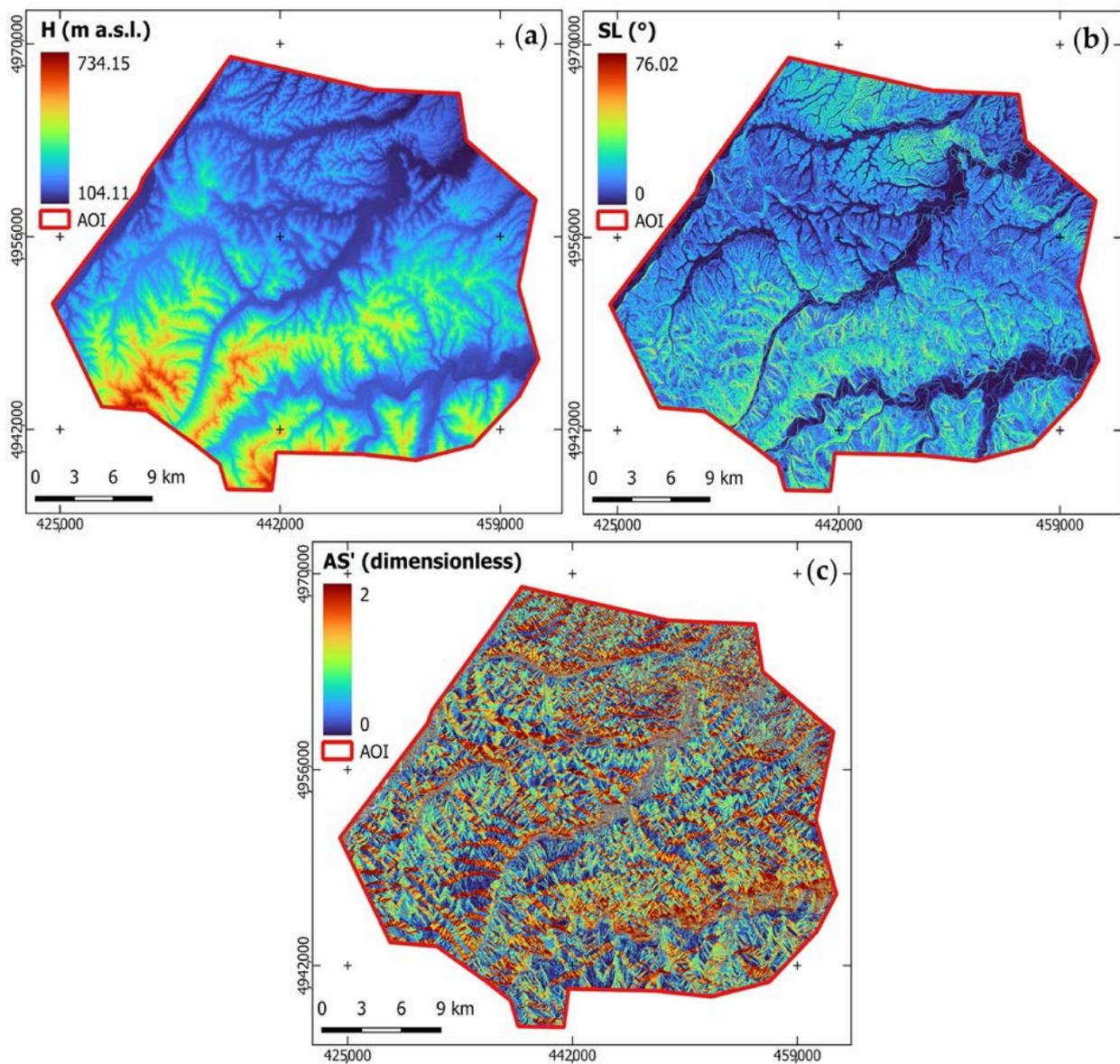
**Figure 7.** Maps of  $H$  (a),  $SL$  (b), and  $AS'$  (c) raster layers in the study area. Reference frame is WGS 84 UTM zone 32N (EPSG: 32,632).
