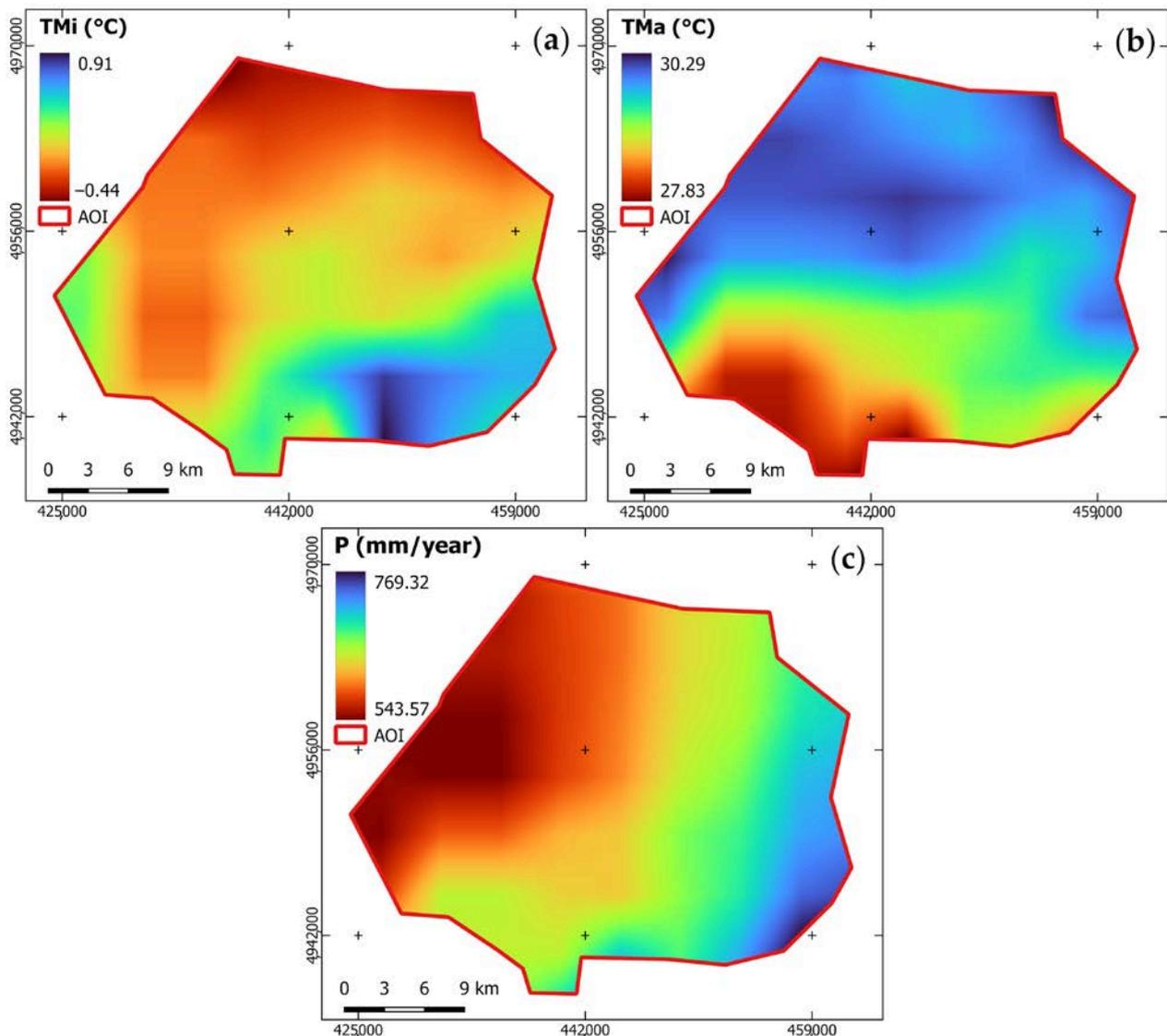
**Figure 6.** Raster layers mapping climatic features in the study area: (a) average yearly minimum temperature ( $TMi$ —°C); (b) average yearly maximum temperature ( $TMa$ —°C); and (c) average yearly cumulated precipitation ( $P$ —mm/year). (EPSG: 32,632, WGS 84/UTM zone 32N).
