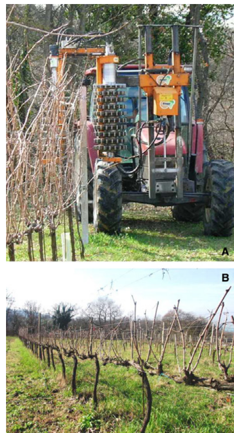
Figure 1 (A) Mechanical prepruner at work in the spur-pruned cordon-trained Sangiovese vineyard, and (B) vines just after the prepruning treatment in winter.
