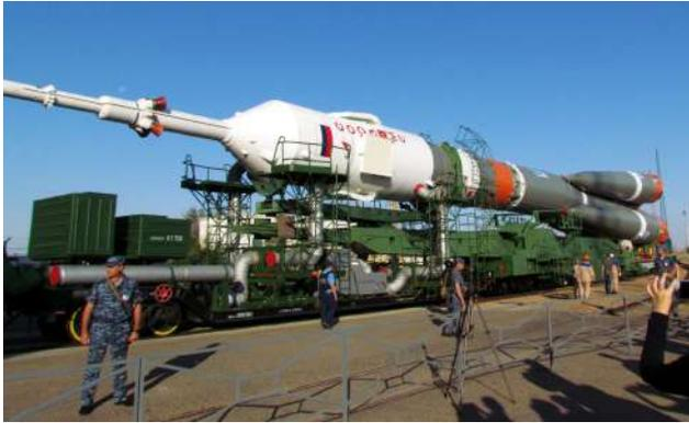
**Fig. 7** The Soyuz-MS14 rocket on its roll-out to the launch pad, 19-8-2019. This was a peculiar uncrewed flight, where a Soyuz capsule (with escape tower visible on the left part of the picture) was used to launch cargo to the ISS. This was to test a new Russian guidance system for the first time without risking a manned flight. In addition to Mini-EUSO, among the cargo was the humanoid robot Fedor.
