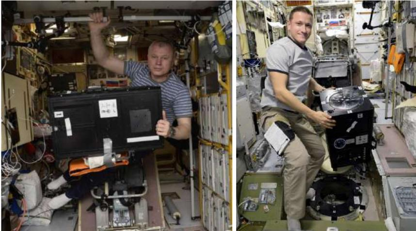
**Fig. 11** **Left:** the cosmonaut Oleg Novitskiy with Mini-EUSO. On the bottom of the picture is visible the pouch with the data cards. **Right:** Cosmonaut Ivan Vagner with Mini-EUSO prior to its installation on the UV transparent Zvezda window (center bottom of the figure). The instrument front lens is visible between the hands of the cosmonaut.
