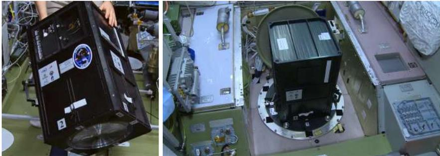
**Fig. 9** **Left:** Mini-EUSO telescope managed by the cosmonaut before to be installed on the nadir-facing UV transparent window of the Zvezda module. **Right:** Mini-EUSO mounted on the UV transparent window. The velocity vector is usually toward the bottom of the picture, in the side marked as '1'.
