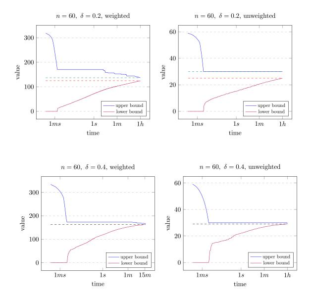
Figure 7: Profiles of the upper bound and the lower bound during the computation on four instances with 60 vertices: the upper row concerns the weighted and unweighted instance 60\_p0.2\_5, with density  $\delta = 0.2$ ; the lower row concerns the weighted and unweighted instance 60\_p0.4\_3, with density  $\delta = 0.4$ .
