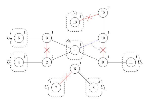
Figure 3: Example of graph manipulations: removing each of the three edges (2,3), (6,7) or (12,13) (in red) or replacing edge (9,10) (also in red) with (1,10) (in dotted blue) yields a relaxation of the original problem.
