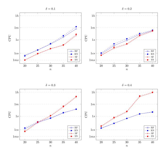
Figure 5: Computational time required by the branch & bound algorithm on the weighted instances of Hosteins (2020), respectively with the refined bound and all fixing procedures (RF), the refined bound and no fixing procedures (RN), the simple bounds and all fixing procedures (SF), the simple bounds and no fixing procedures (SN)
