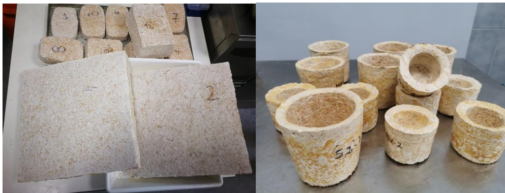
Fig. 1. Fabricated mycelium composites
