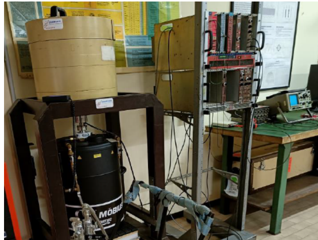
Fig. 4.5.: Image of the HPGe used for this work. On the right of the detector, the readout electronic and the connection with the acquisition pc can be shown.
