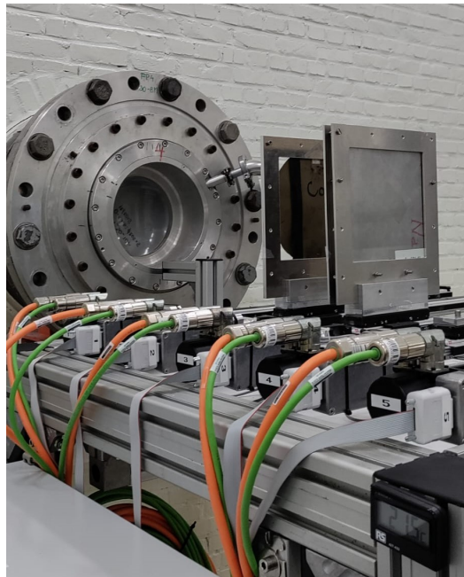
Fig. D.10.: Picture of the Na and Co filters used for the background estimation through the black resonance technique [151].
