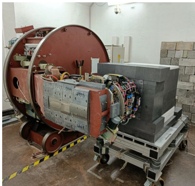
Fig. 2.19.: External image of the e-LiBaNS facility. The grey structure is the thermal photoconverter.
