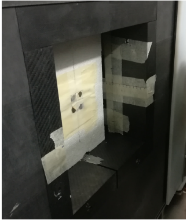
Fig. 5.1.1: ^{197}\text{Au} foils positioned in the e-LiBaNS thermal cavity during the measurement. Two couple of foils are exposed simultaneously around the centre of the cavity.
