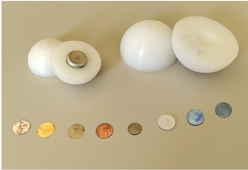
Fig. 5.4.: Picture of the two different NCT-ACS geometries. On the left the 20 mm configuration with the Cd cylinder is reported, while on the right the 28 mm option is shown. On the bottom the activation foils are also displaced, from left to right: In, Au, Mn, Cu, V, NaCl, Re, W.
