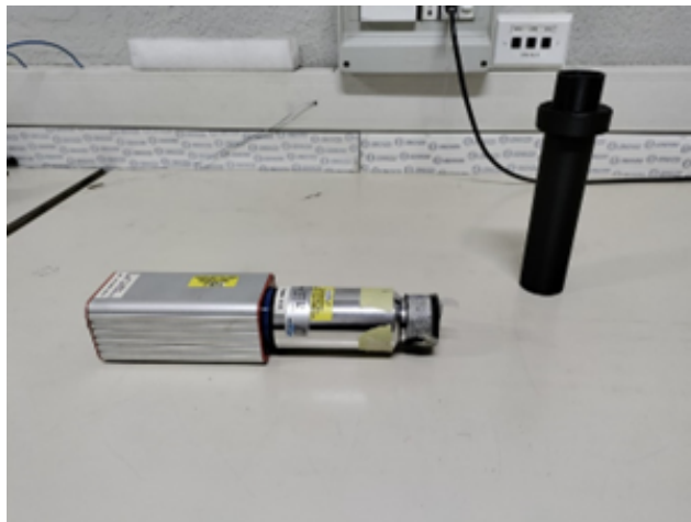
Fig. 7.2.: Picture of the LaBr detector with the "contact" holder inserted on the aluminum end-cap. On the right the "distance" holder can be seen.
