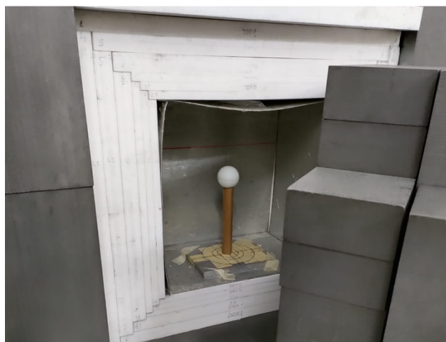
Fig. 5.5.: Picture of NCT-ACS on top of the holder in the irradiation position. The cavity volume is 30 \times 30 \times 20 \text{ cm}^3 . On the right the cavity cap is visible.
