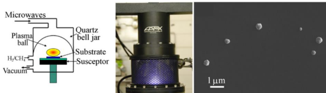
Figure 17 CVD example growth of nanodiamonds with embedded SiV color centers [132]
