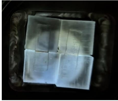
Figure 71 Picture of the luminescence produced by the ion beam on Cesium hydride in the exit of the source.
