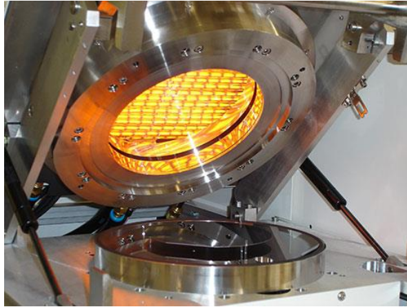
Figure 53 RTA processing chamber[255].
