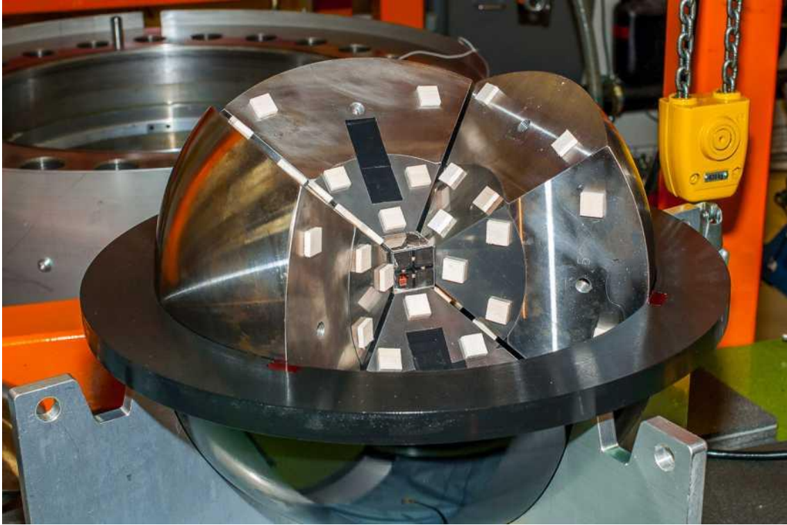
Figure 54 Mult anvil HPHT press [258].
