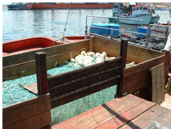
Fig A2.11. Multifilament mainline and hooks in stern of artisanal longline vessel.
