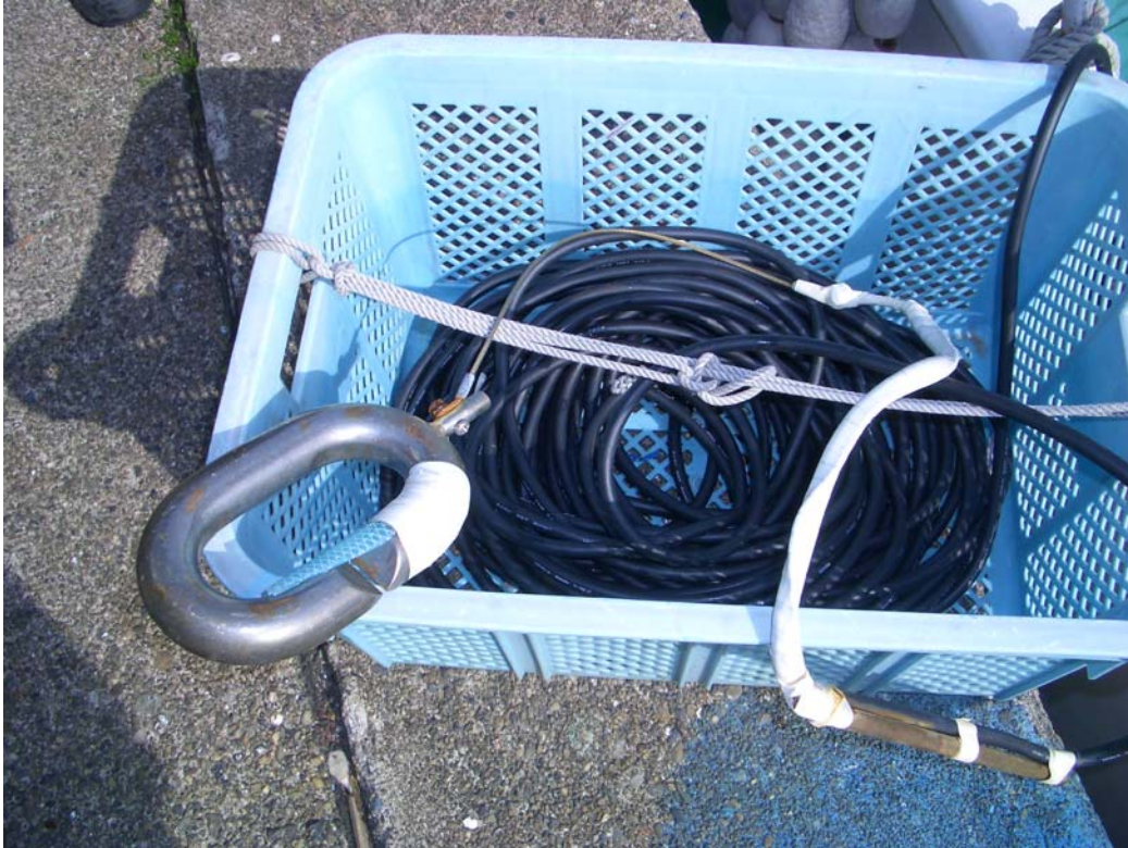
Fig. A5.10. The ring and electrical cord of the "shocker" device used by engan fishermen based in Kii-Katsuura to immobilize sharks. (Photo: T. Miyamoto).
