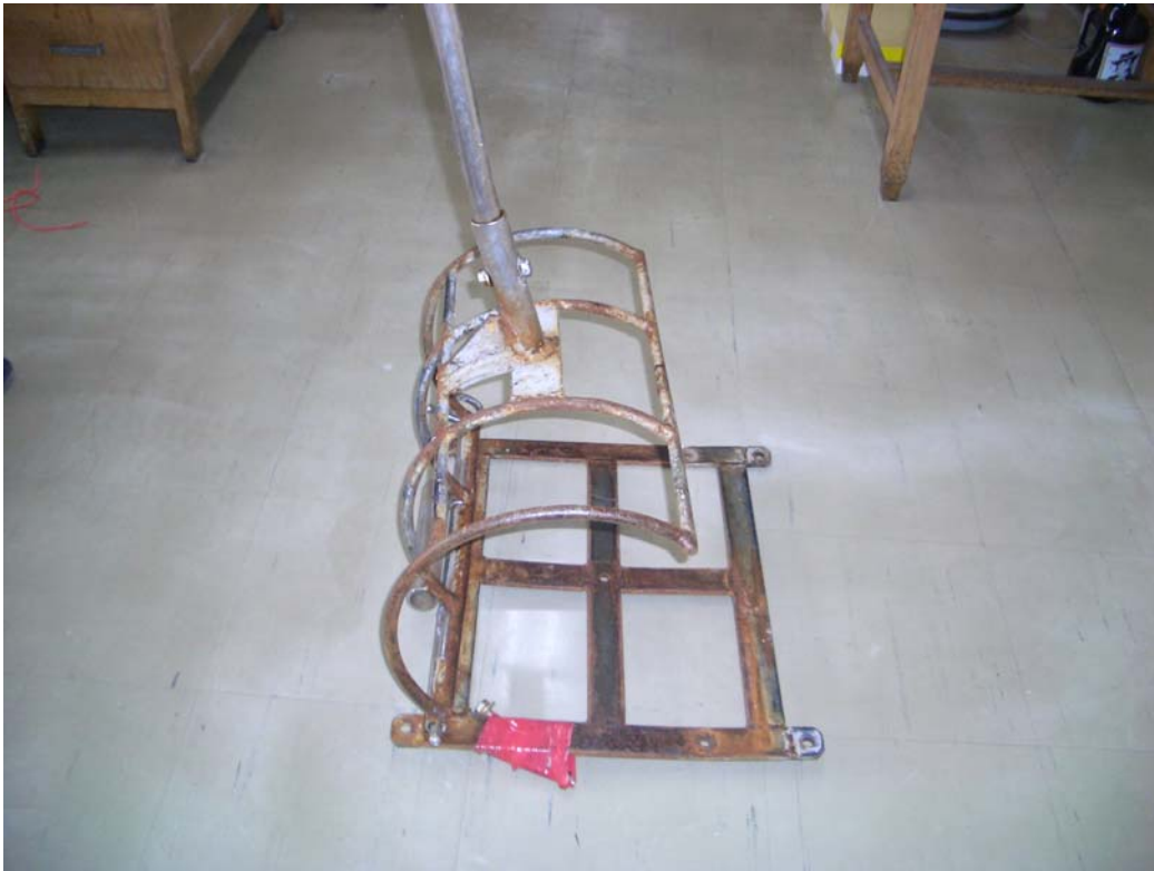
Fig. A5.8. Clamping device designed and used by one kinkai fisherman based in Kesenuma for immobilizing sharks (photo courtesy of T. Miyamoto).
