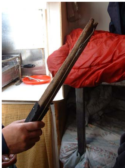
Fig. A2.10. Fisherman demonstrating an improvised de-hooker.
