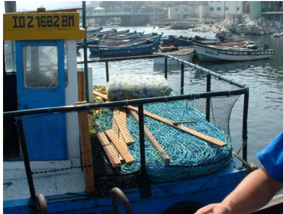
Fig. A6.7. View of a multifilament longline of an artisanal vessel.
