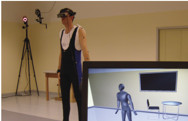
Figure 1. Subject wearing the HMD and markers was immersed in the movement analysis laboratory and consequently represented in the virtual laboratory.
