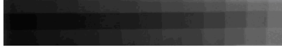
Fig. 9: INES neutron radiograph of a step wedge made of (from top to bottom) brass, iron and bronze.
