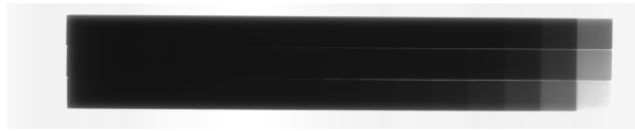
Fig. 13: X-ray radiograph of a step wedge made of bronze, brass and iron (top to bottom).
