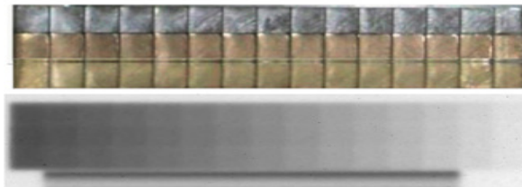
Fig. 5: Iron (T), bronze (C) and brass (B) step wedges: photo and NECTAR neutron radiography.
