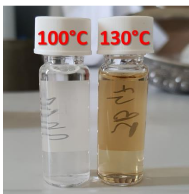
Figure 19: Resin degradation phenomena during the reaction conducted at 130°C
