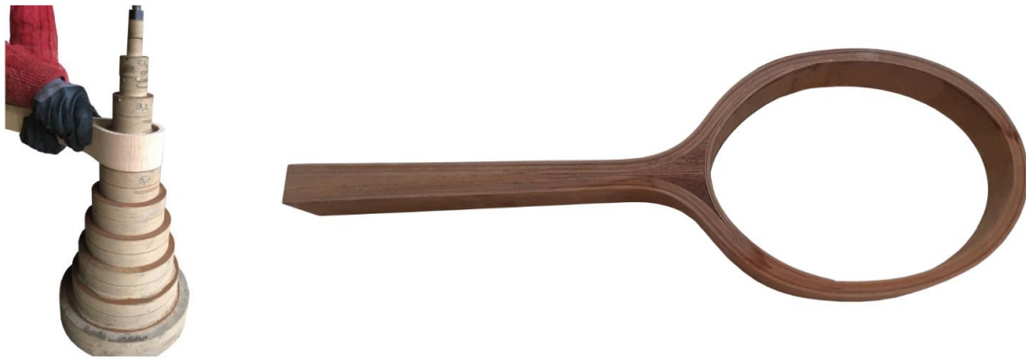
FIGURE 11.1 Left: device used to test the flexibility of plywood and veneers. Right: multiple-layered raw blocks were assembled, cut, and finished to obtain the final wood laminate rackets (images, not to scale, R. Zanuttini).
