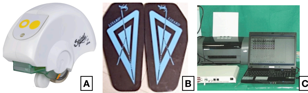
Fig. 1.3.5.: Non invasive postural devices used for protocol test in University of Turin: Spinal Mouse (Idiag, Volestwil, Switzerland) (a), Lizard Stabilometric Platform (Lizard, Lemax s.r.l., Como, Italy) (b), K7-I Kinesiograph (Myotronics, Tukwila, WA, USA) (c).
