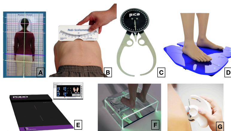
Fig. 1.3.3.: Non invasive postural devices: Scoliometer (a), Inclinometer (b), Goniometer (c), Stabilometric platform (d), Baropodometric platform (e), Podoscope (f), Spinal Mouse (f).
